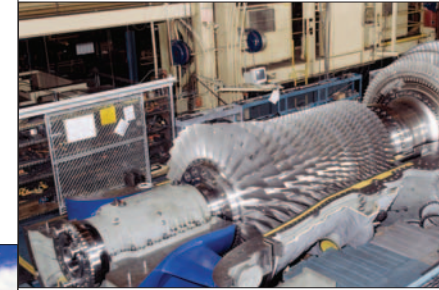
This MS9001FB is seen on half shell during assembly.
