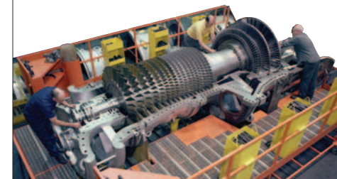
An MS6001B rotor is seen on half shell.
