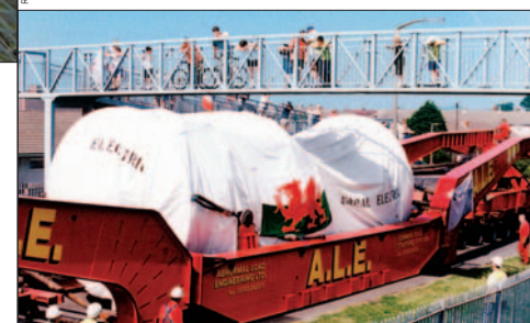
World's first H turbine is transported through Wales to Baglan Bay Power Station.
