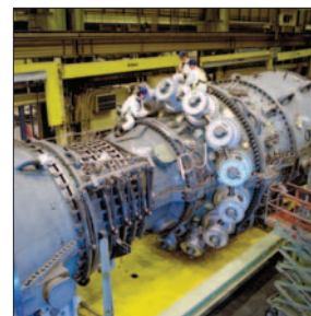
A 9H gas turbine is readied for testing.
