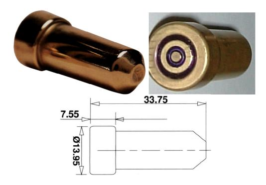
The rearming cartridge allows multiple in-flight recocking, up to six times in the DEFA 554 and DEBO-30-M2 cannons and up to two times in older models (552 / 553 / Mk164) in case that a cartridge of ammunition in the revolver chamber misfires for any reason (faulty primer or other reasons).
