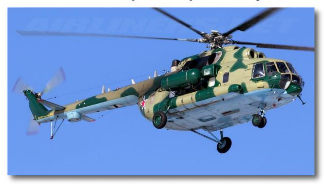
• The Mi-8 is a transport helicopter of Soviet origin. It was developed in the early 1960's to provide Soviet forces with a larger capacity helicopter than the Mi-4 and more maneuverable and practical than the Mi-6. The commonly used NATO reporting name is Hip. The Mi-8 and the second generation Mi-17 are some of the most numerous and widely exported helicopters ever built. Besides its troop transport role it can be used as an attack helicopter due to its significant weapon load.
