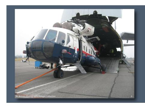
The Mi-8 and Mi-17 have the ability to carry 24 troops or 12 stretchers or 4 t of cargo. It is also possible to carry 3 to 4.5 t of cargo on a sling below the aircraft.
