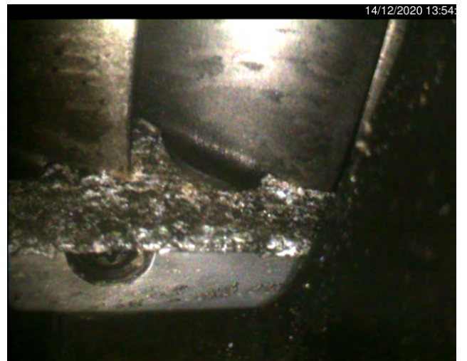
Picture 4: stage 1 shrouds, deposits
