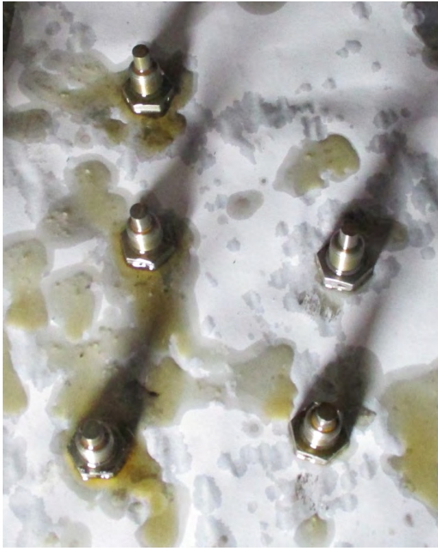
Picture 51: chip detectors and screens clean. No remarks.
