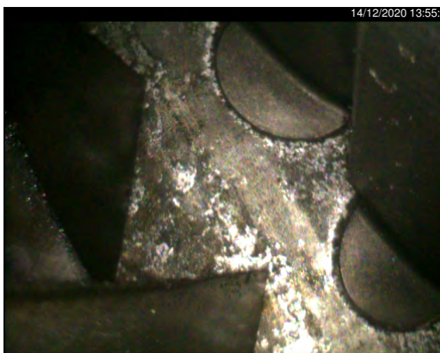
Picture 5: stage 1 shrouds, salt and deposits
