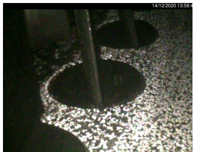
Picture 6: stage 1 shrouds, salt and deposits
