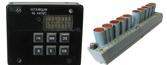
Set of IR decoy dispenser system and radar chaffs
