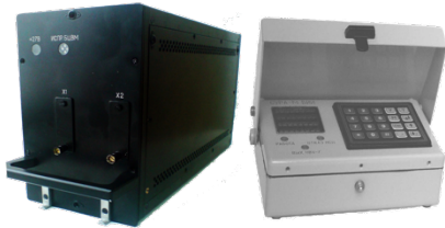
Ballistic computer set VDK-558 for aircraft weapon control system upgrade
