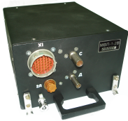
Air data unit MVP-1 for aircraft weapon control system upgrade
