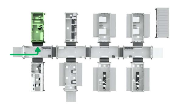
This department, built on a 20ft container, is specially designed for conducting radiology tests in field hospitals. The container is divided into two rooms. The X-Ray machine is located in a specially coated room, while the other room is designated as a waiting area for patients and an operator room.
