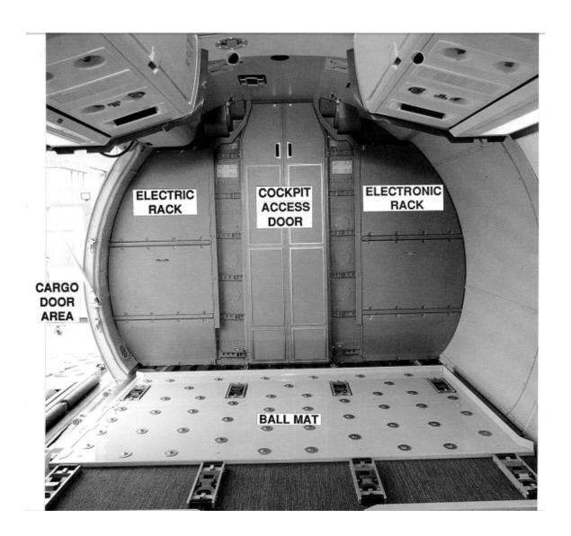
Ball mat consists of freely rotating balls located in housings and protuding above surrounding surfaces.
